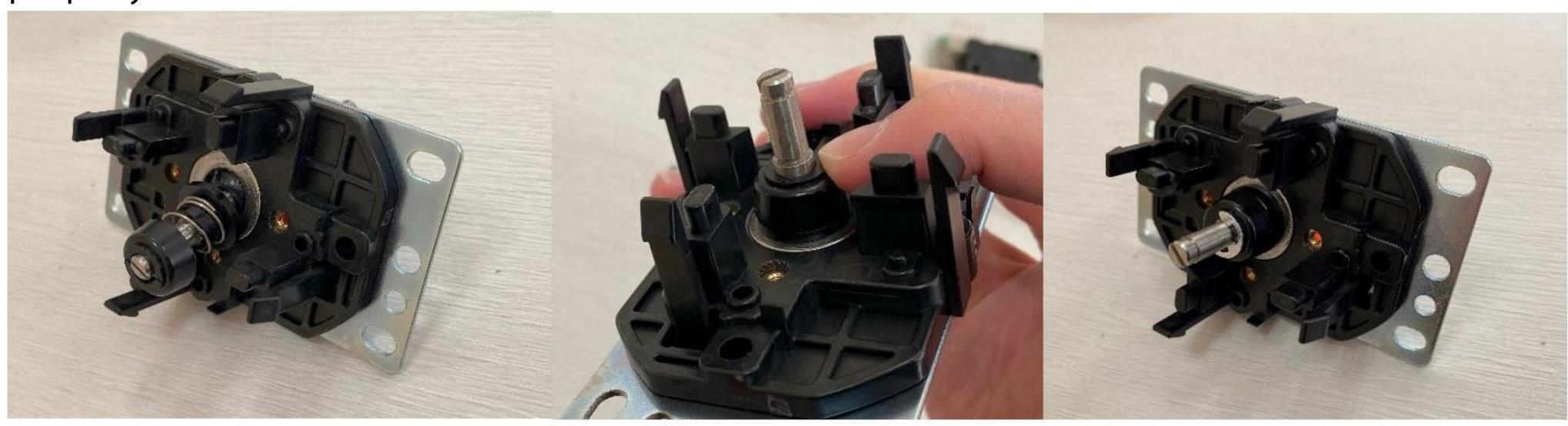
5. Install the washer (#3), rubber bearing (#2), and another washer (#3) in sequence.
